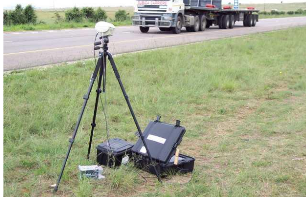
Picture 1: Complete MonCam installation at the side of the road.
