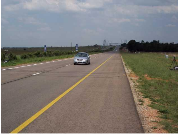
Picture 2: Two MonCam installations one on each side of a carriage way
