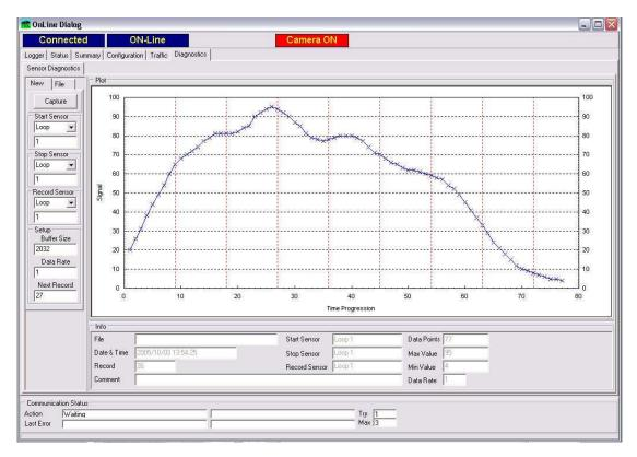
A typical sensor response of a light vehicle over a loop.
